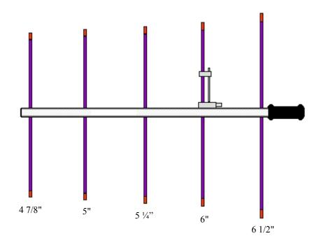
5 Element Portable Antenna for 70 cm
