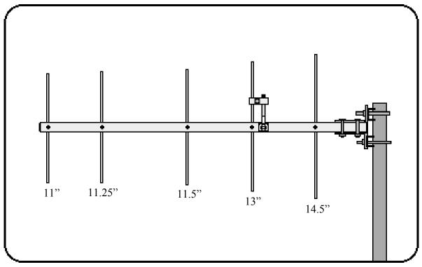
This antenna must be end mounted with the M/B Mounting Bracket included.
