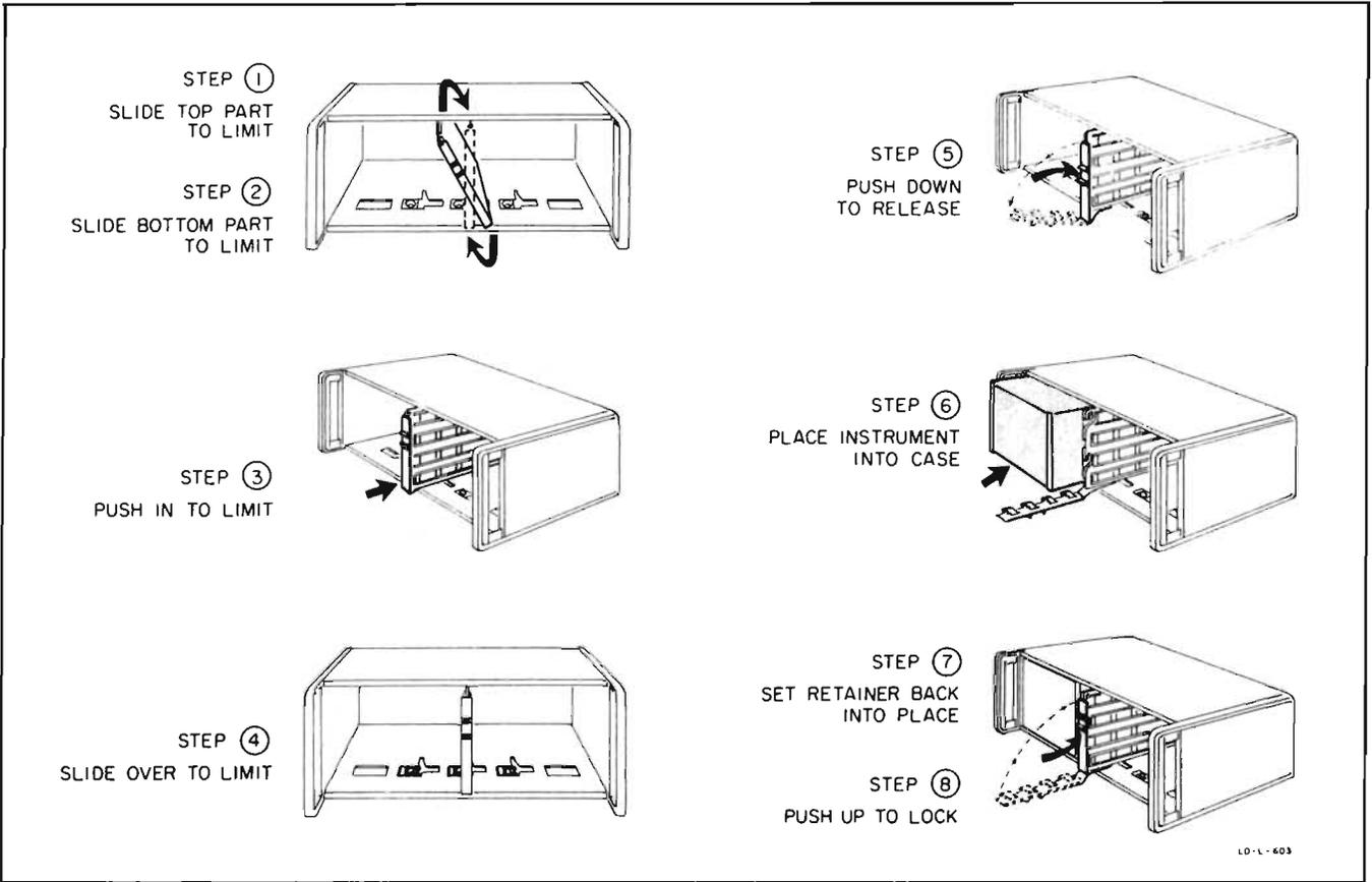
Figure 2-2. Steps to Place Instrument into Combining Case
