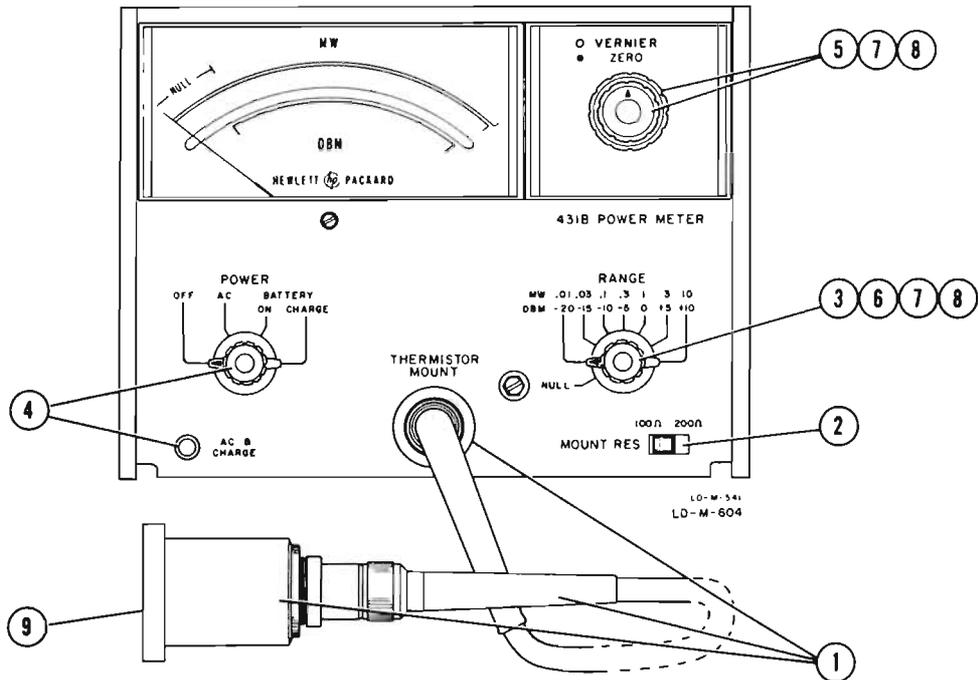
1. Connect thermistor mount and cable to the THERMISTOR MOUNT.  $\oplus$  thermistor mounts and their frequency ranges are given in table 1-2, Model 431B Thermistor Mounts.
