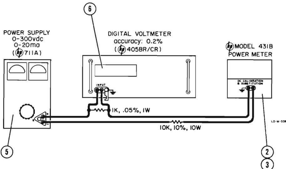
1. With power supply turned off, connect the Model 431B as shown above.
