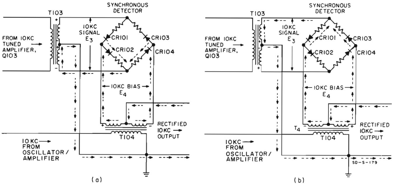
Figure 4-5. Synchronous Detector
