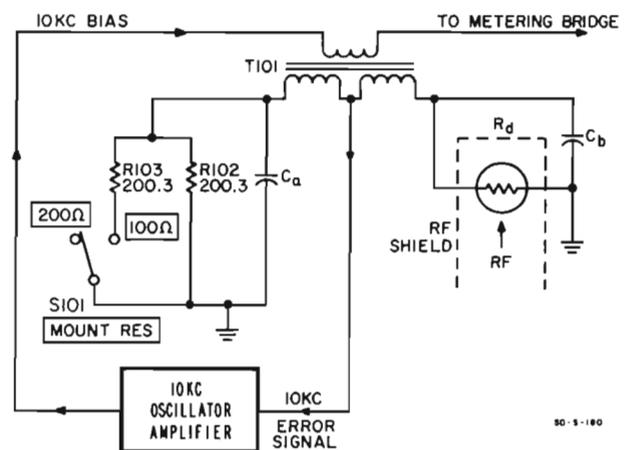
Figure 4-2. RF Circuit
