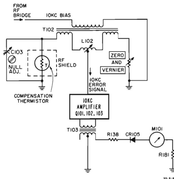
Figure 4-4. Nulling Circuit
