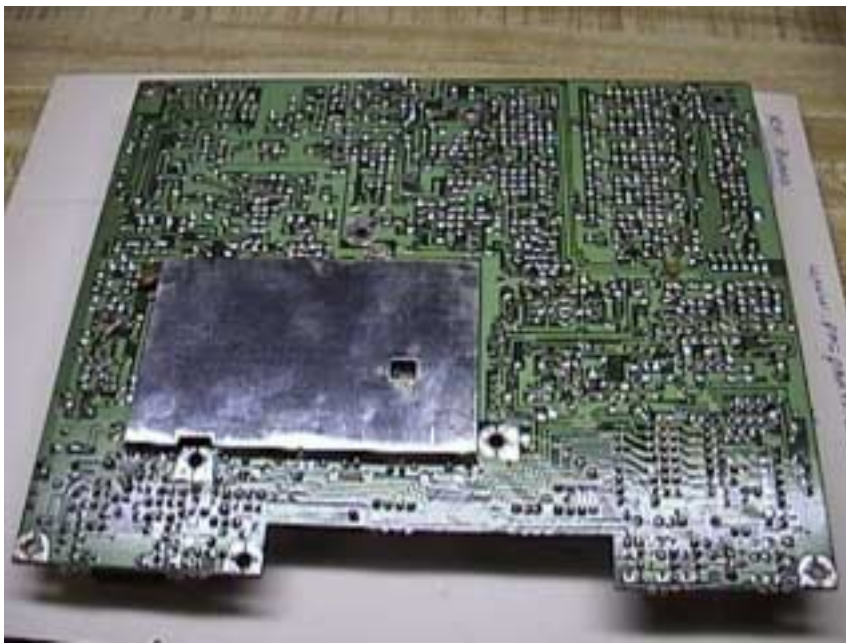
RF board removed (solder side) with shield.
